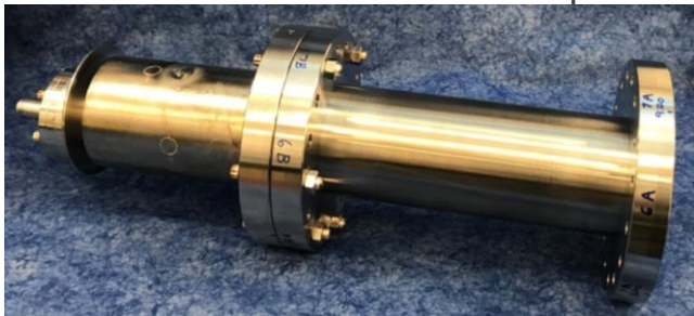
Test box can with HHOM coupler
