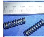
20 titanium G5 springs (total prestress: ~360 N)
