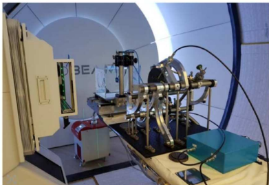
Setting the standard: NPL's portable calorimeter provides a more accurate reference point for proton-beam dosimetry. (Courtesy: NPL)
