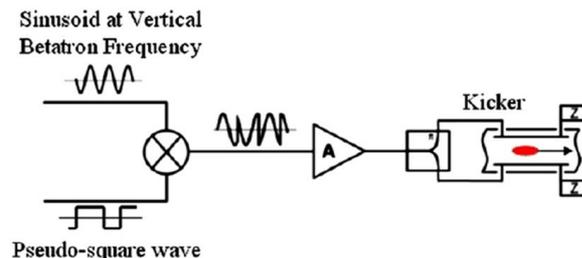
Fig. 1. Basic scheme for the new cleaning technique.
