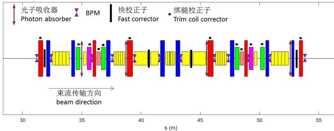
HEPS lattice is 24 cells which have two 7BAs structure, in every 7BA, there are 10 BPMs in arc and 2 BPMs in ID, so totally we have  $48 \times 12 = 576$  BPMs.
