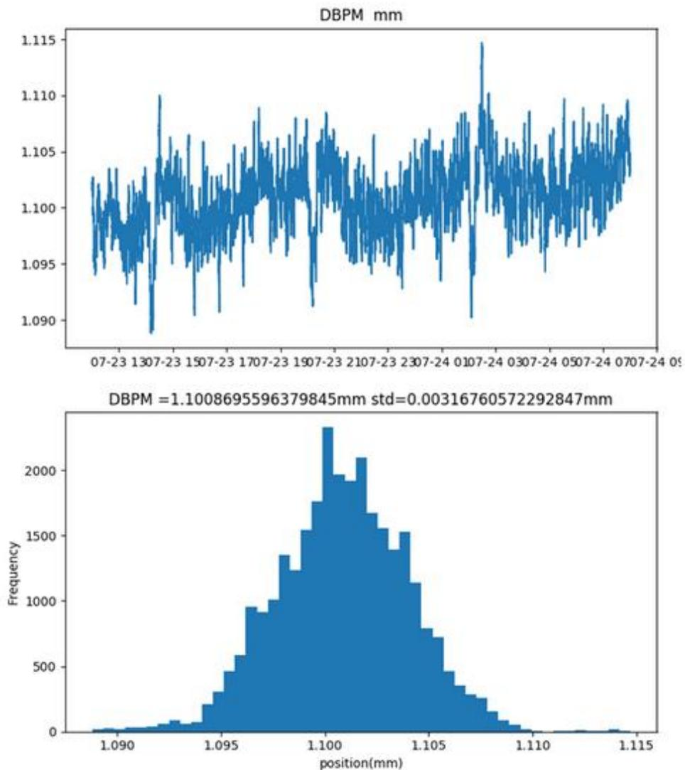
The beam position resolution results for the IHEP-developed DBPM (Image by IHEP)
