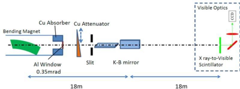
Imaging system based on KB mirrors
