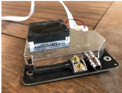
SDS011: A better PM2.5 and PM10 detector
