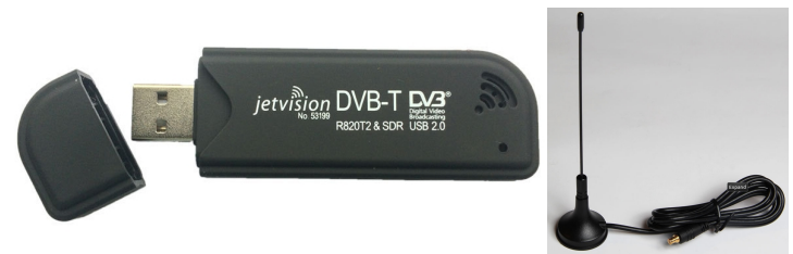
ADS-B receiver: follow aircraft over my town. Maximum range: ~58 nm with low-cost antenna
