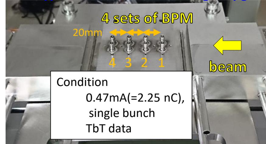
If gain balances are properly corrected, 4 BPM readings come close to one point.
