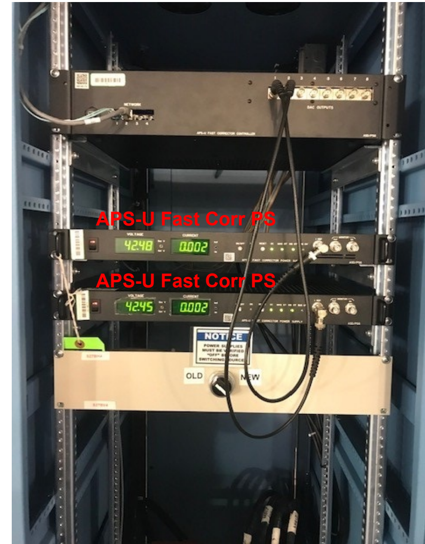
APS-U Prototype Fast Corrector PS Cabinet
