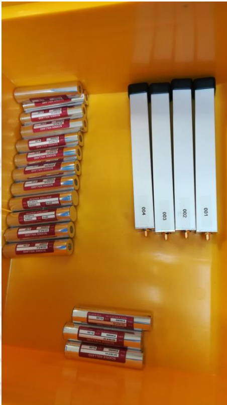
Scintillators and first assembled BLM
