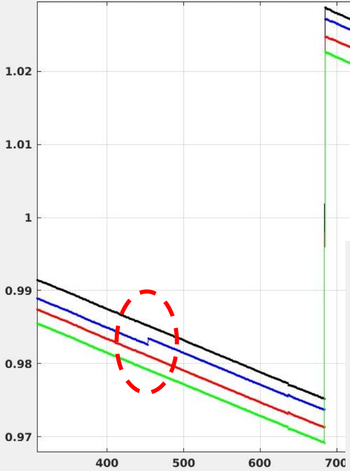
May 6, C14, Spark-2, a jump of 2um, caused by Ch.B (blue)
