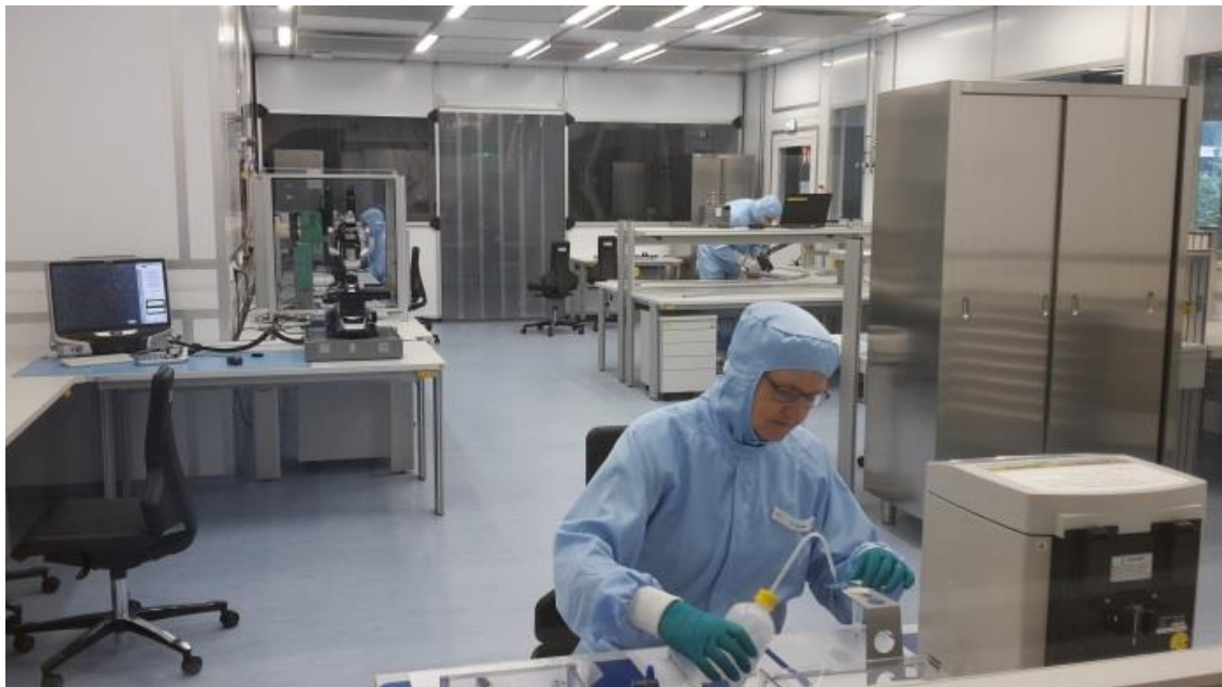
View of the CMS area of the DAF cleanroom at DESY, with microscopes and automated module assembly system. All major devices have been installed and are being commissioned.
