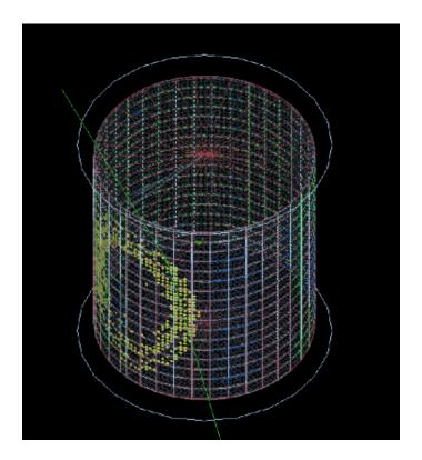
An open-source, GEANT4-based simulation code for water Cherenkov detectors
