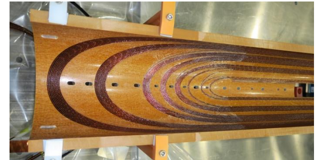
Coil after curing
