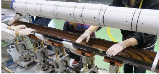
4. QPH, insulation wrapping
