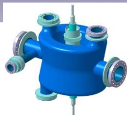
Double Quarter Wave (DQW) cavity at ATLAS (V)
