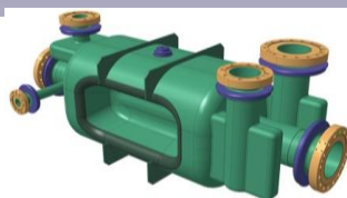
RF-Dipole (RFD) cavity at CMS (H)
