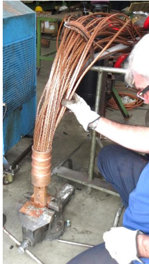
Cable bundle braised on the lug: WCC with spring (BRAR, 2000mm 2 )
