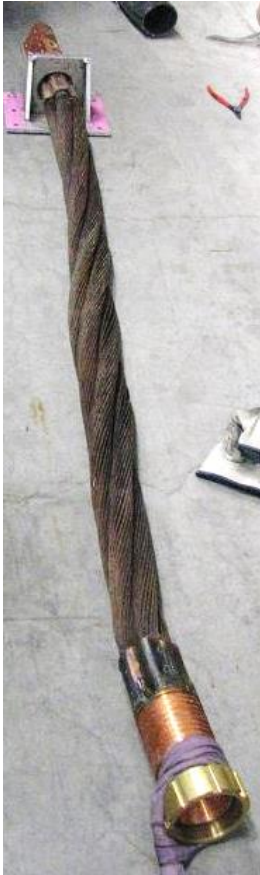
Cable bundle crimped on the lug: WCC without spring (FLOHE, 2000mm 2 )
