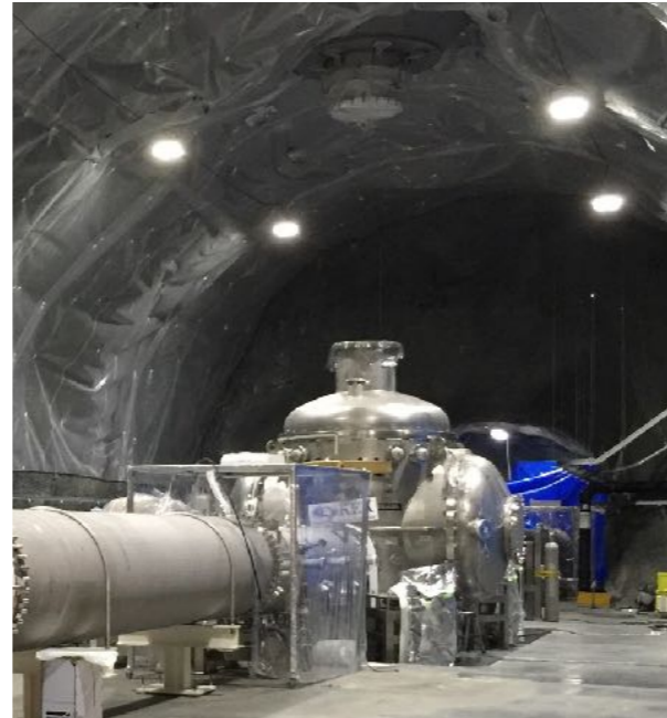
Cryostat for a sapphire mirror (not connected to the 2nd floor) Achieved pressure 10^{-5} Pa in cryogenic to 10^{-4} Pa in room T.
