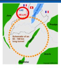
Also studied: HE-LHC: √s=27 TeV using FCC-hh 16 T magnets in LHC tunnel; L~1.6x10<sup>35</sup> → 15 ab-1 for 20 years operation
