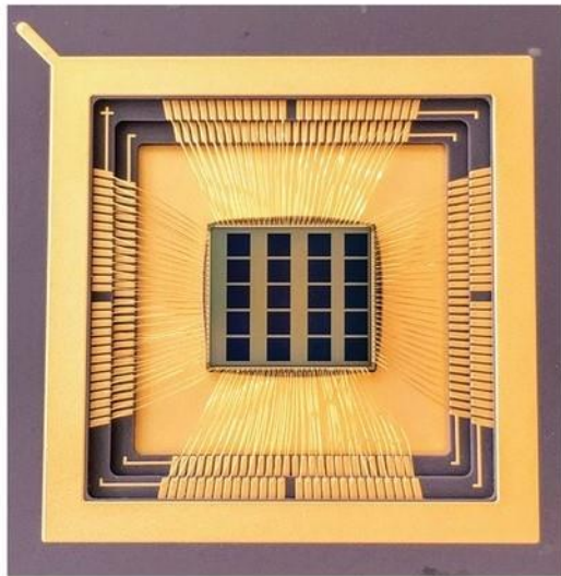
FIGURE 2. A Dartmouth QIS test chip contains 20 different 1 Mjot QIS arrays and was fabricated by TSMC in a modified 45/65 nm 3D-stacked BSI CIS process.
