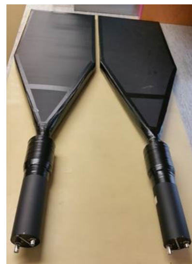
Beam Trigger (2 pairs of scintillators)
