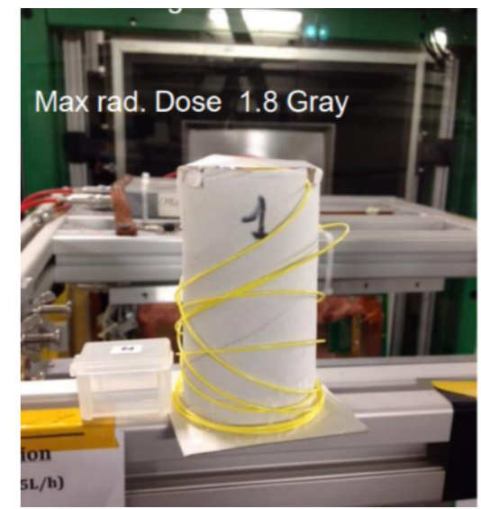
microlens and optical fibres for the TOP PID detector of Belle II experiment
