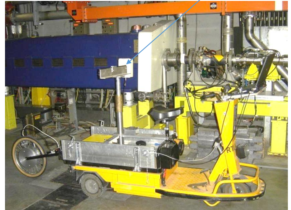
Measuring probe Plastic scintillator Vol: 200cm 3
