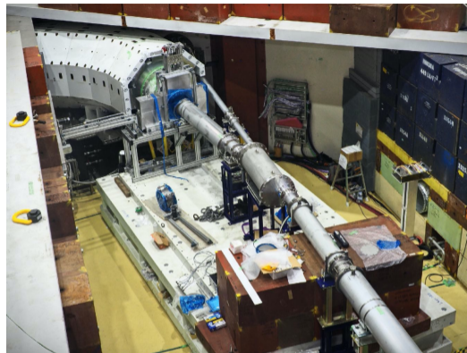
Figure 11: COMET Muon solenoid and beamline [12]
