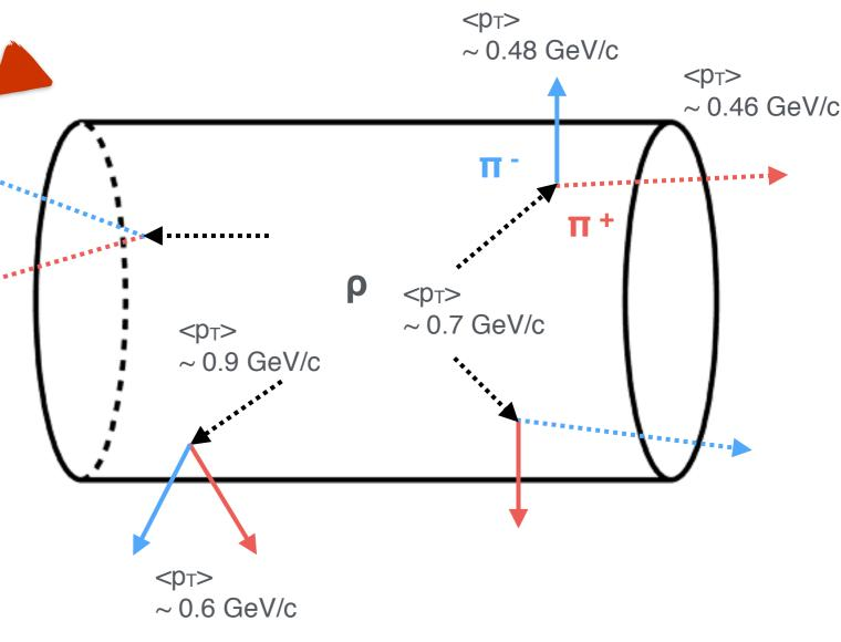
reported by the CMS experiment (~0.12). One can narrow down the  $p_T$  coverage to reduce such a  $p_T > -A_{ch}$  dependence. When changing the  $p_T$  upper limits from 5 to 0.5 GeV/c, the slopes get reduced to ~0.01 (by 1/10). Therefore, it is important to perform the measurements of  $v_2$  at the narrow  $p_T$  range to eliminate the LCC effect as low as possible.
