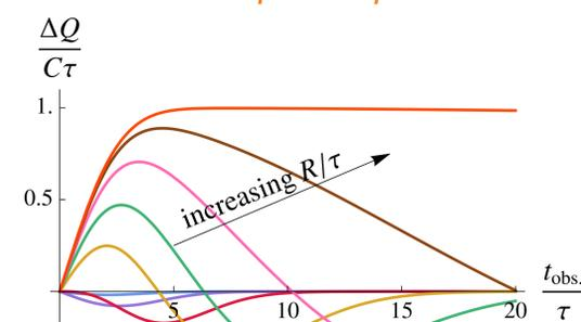
$$\frac{\Delta Q(t_{\text{obs}}, \tau, R)}{C\tau} \rightarrow \begin{cases} \text{erf}\left(\frac{t_{\text{obs}}}{2\sqrt{2}\tau}\right) & \text{large } R \\ e^{-\frac{t_{\text{obs}}^2}{4R^2}} \left(1 - \frac{t_{\text{obs}}^2}{4R^2}\right) & \text{small } \tau \\ \frac{1}{\sqrt{2\pi}} \frac{(R/\tau)^2 - 1}{((R/\tau)^2 + 1)^2} \frac{R^2 t_{\text{obs}}}{\tau^2} + \mathcal{O}((t_{\text{obs}}/\tau)^2) & \end{cases}$$
