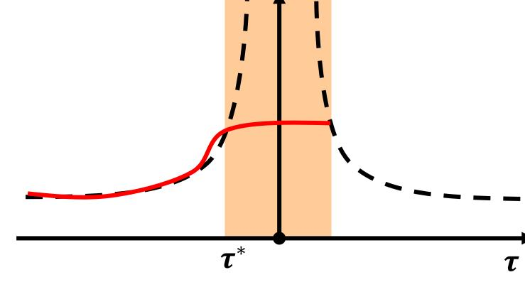
• For the system cools down to the critical point, the relaxation time  $\tau_{rel}$  diverges due to the critical slowing down. After the point  $\tau^*$  where  $\tau_{rel} \simeq \tau_{quench}$ , the system becomes out-of-equilibrium and the typical scales fixed:
