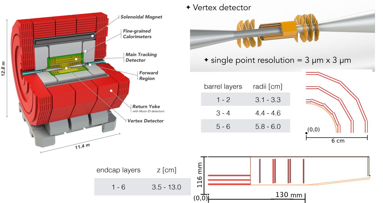
+ Stub length O(cm) => in this study, the CLICdet has been reduced to the vertex detector only
