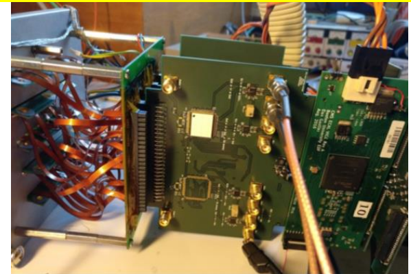
Analog test setup at Saclay for ECAL VFEDs
