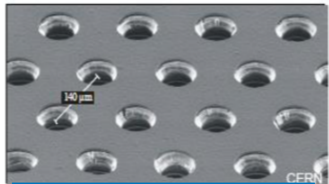
Electron microscope photograph of a GEM foil
