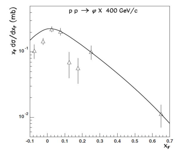
Experimental data on  $x_F$ -spectra of  $\Phi$ -mesons in pp collisions at 400 GeV/c (LEBC-EHS Collaboration), compared to the corresponding QGSM results.
