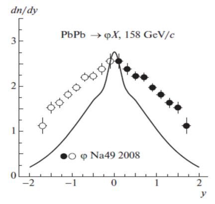
Experimental data on the y dependence of the inclusive density for  $\Phi$ -meson production, dn/dy, in Pb-Pb collisions at 158 GeV/c, compared to the results of the corresponding QGSM calculations.
