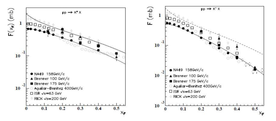
Experimental data on the invariant cross section of  $K^+$  and  $K^-$  in pp collisions at different energies, compared to the corresponding QGSM results.
