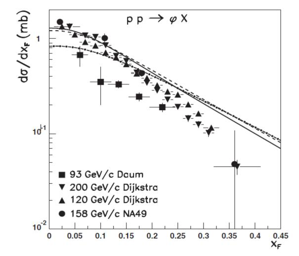
Experimental data on  $x_F$ -spectra of  $\Phi$ -mesons in pp collisions at 93, 120, 158, and 200 GeV/c, compared to the corresponding QGSM results at 93, 158, and 200 GeV/c.
