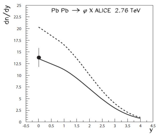
QGSM prediction for the rapidity dependence of the density for  $\Phi$ -meson production, dn/dy, in central Pb-Pb collisions at  $\sqrt{s} = 2.76 TeV$ , with (full) and without (dashed curve) inelastic shadowing, compared to the ALICE experimental point.
