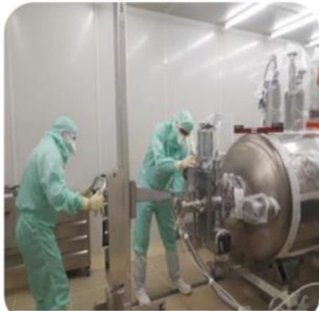
Assembly of new pumping crosses
