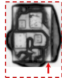
Figure 3: SAM image after 300 thermal cycles [1].
