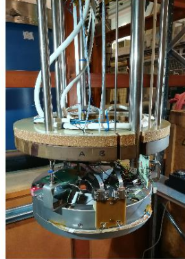
Magnet connected to mechanical support and electrical link to bus-bars. Coil ends are soldered with a MgB_2 -NbTi junction on a PCB glued on the lower coil's face.
