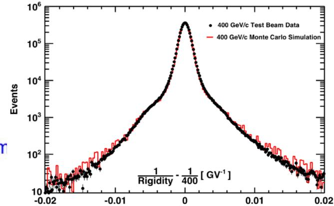
*Error in  $1/\text{rigidity}$  for 400 GeV test-beam protons.*
