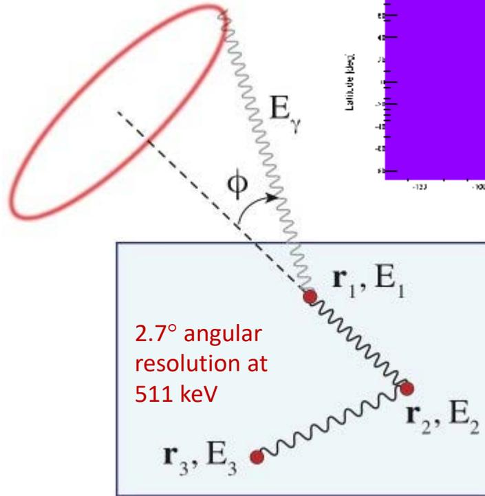
Two successive Compton scatter give information needed to reconstruct a circle on the sky. Redundant information from scattering energies allows the interaction order to be inferred.
