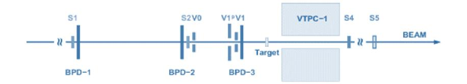
Beam Position Detectors (BPD-1,2,3) provide position and charge measurement of the incoming beam particles during the data taking. The upgrade of BPDs is necessary
