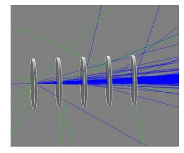
1500um thick carbon targets (5mm radius, 15mm spacing)
