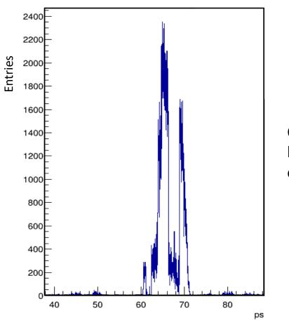
Coincidence results of Sr90 between two layers positioned only 10mm apart.
