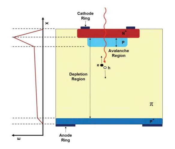
Standard n+ implant is typical for silicon diode detectors.
