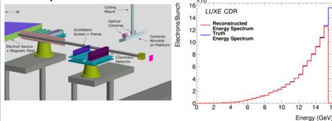
GEANT4 rendering of the electron detection subsystem
