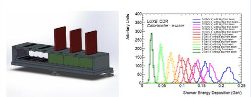
CAD model of electromagnetic calorimeter
