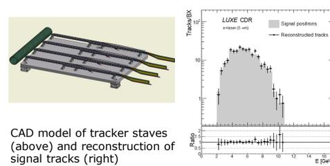
CAD model of tracker staves (above) and reconstruction of signal tracks (right)
