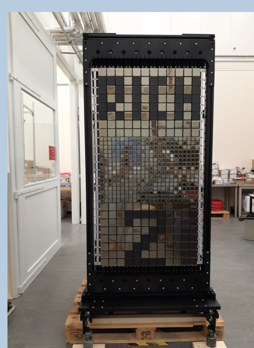
Figure 7: RICH2 A side commissioned. On the right, hitmap obtained with the front end electronics switched on and CLARO channels triggered by noise.
