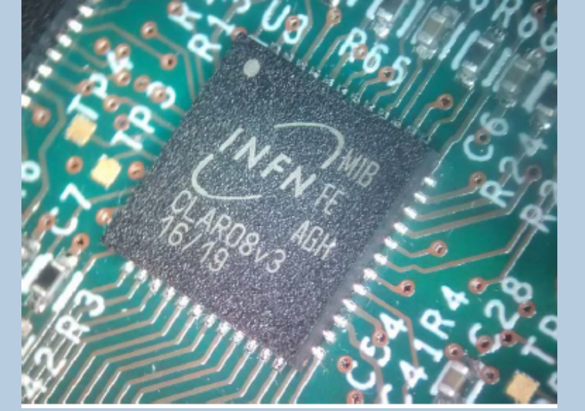
Figure 4: Left: front view the two types of MaPMTs. Right: the CLARO ASIC
