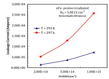
➤ Leakage current increases with fluences at 293 (RT), and 297 K (Rt+4K) that shows the experimental results a per (3)
