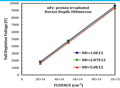
➤ Hamburg Penta Trap Model (HPTM) model can reproduce the experimental data in n, p, here we used in 300 μm n-Fz proton irradiated Si strip detector as shown in (1), V<sub>fd</sub> estimated from SRH calculations (2) and decreases with increasing doping concentration
