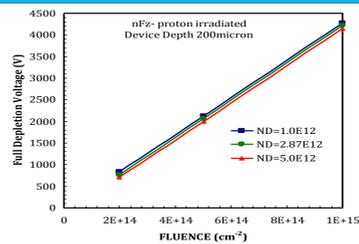
➤ HPTM model can be used to get V<sub>fd</sub> in 200 μm n-Fz proton irradiated Si strip detector, 50% less V<sub>fd</sub> have been obtained in 200 μm n-Fz proton irradiated Si strip detector than 300 μm strip detector irradiated by protons
