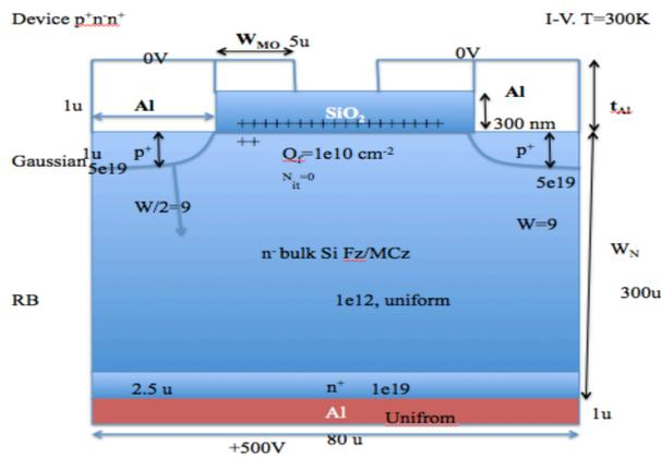
➤ Cross-section of the 0.0625 cm<sup>2</sup> x 200/300 μm n-Fz/n-MCz Si strip detector /PAD diodes used in the present study for SRH calculations and TCAD device simulation
