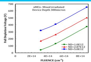
➤ V<sub>fd</sub> increases with the mixed irradiated fluences for the three doping concentrations in thick n-MCz Si strip detector, less full depletion voltage obtained than other n-Fz proton radiated detectors, less V<sub>fd</sub> observed due to the compensation of the deep traps in n-MCz as compared to n-Fz Si strip detector
