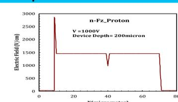
➤ Less E-field at curvature of junction and in the base region of the detector, and also less E-field at E-field gutter than mixed irradiated n-MCz Si Strip detector
