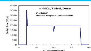
➤ With an increasing mixed doses, E-field at curvature of junction saturates and at E-field gutter, X=40 μm too
