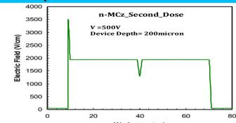
➤ E-field increases at curvature of junction and slightly increase at E-field gutter, X=40 μm
