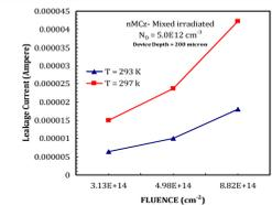
➤ Leakage current increases with fluences at 293 (RT), and 297 K (Rt+4K) that shows the experimental results as per reference (3)
