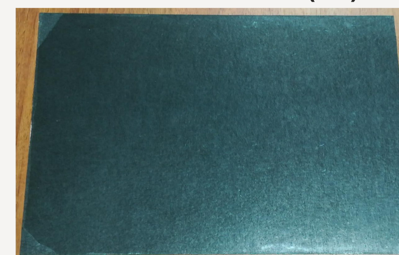
Sandwiched Carbon Fiber sheet 200 mm x 290 mm x 0.3 mm fabricated at St Petersburg State University [6] Image Courtesy [5]
