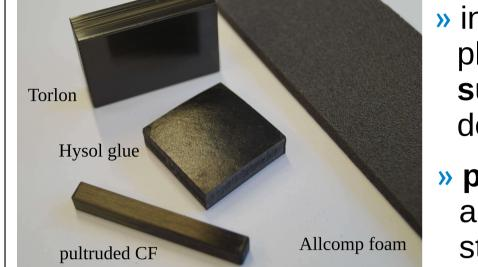
» investigate various materials planned for the use in the **local** supports of the ATLAS ITk detector with **unknown X**<sub>o</sub>
