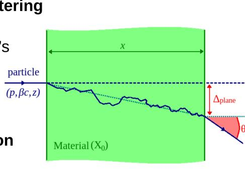
» minimizing the material budget is important factor in the **design of tracking detectors**  $\rightarrow$  e.g. in the design of the new phase-2 ATLAS Inner Tracker (ITk) [1]
