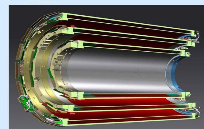
It is a Gas Electron Multiplier (GEM) made by three independent, coaxial tracking layers, each with three multiplication stages.
