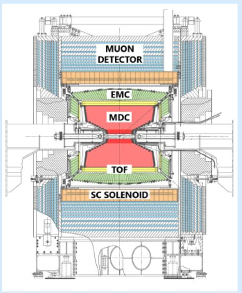
The spectrometer is made up of 5 detectors:
