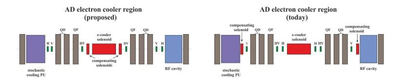
The main difference between two schemes is that with new cooler in AD compensating solenoids are placed right on sides of the main solenoid. The coupling compensation will be local which makes machine operation much more comfortable and provide conditions for better performance
