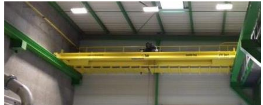
Double girder crane Capacity: 3.2 tonnes Span: 8.360 mm Example of crane «G»
