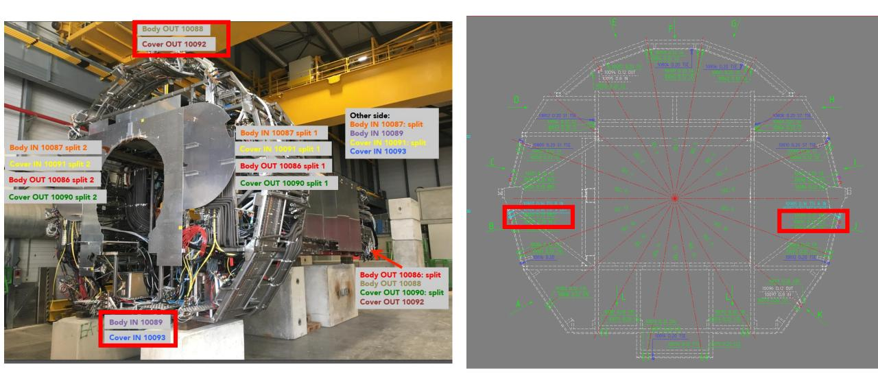
• add 3 tube for Heat exchanger. All 3 of these "new" multilayer pipes have the same size, like for example pipe 10051
