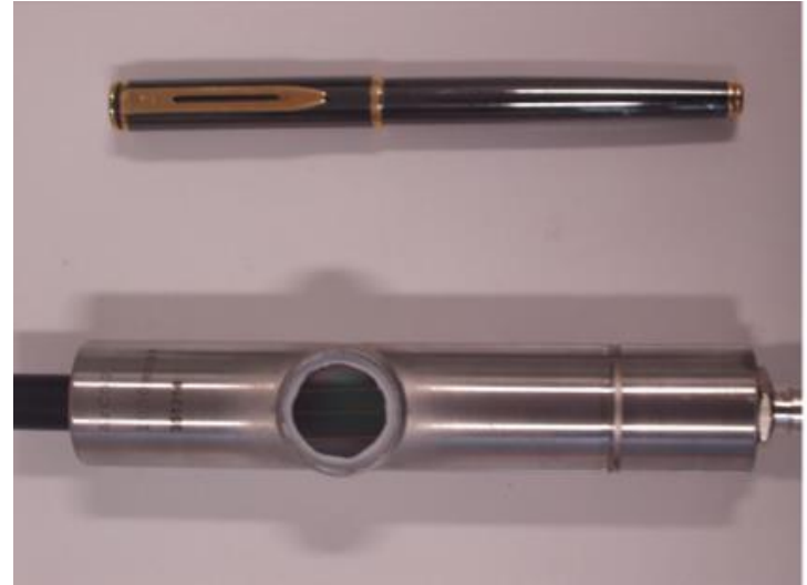
Current flame detector by CERN
