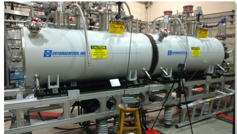
The electron beam ion source EBIS can produce virtually any desired ion species including polarized ^3\text{He}
