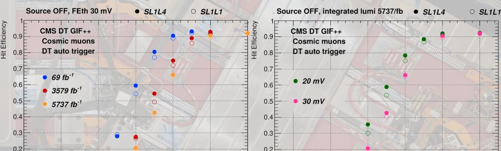
The drop of efficiency for a front-end threshold (FEth) value of 20 mV and high HV values is of the order of a few %.
