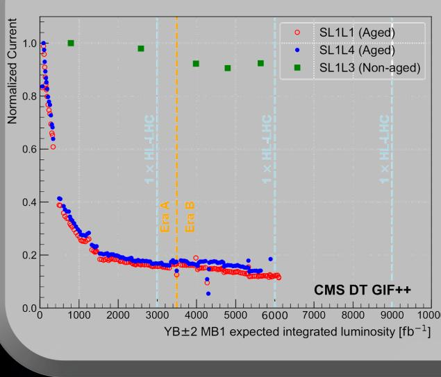
The currents in the aged layers (SL1L1, SL1L4) were monitored during the irradiation period. The currents on the non-aged layer SL1L3 are used as a reference. Most of the drop of currents is observed during the first 1000 fb<sup>-1</sup> of accumulated luminosity.
