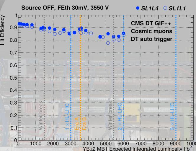
The hit efficiency was weekly measured with no background (source off) during the irradiation of the chamber. For a HV of 3550 V, the hit efficiency is reduced <10% after integrating 2xHL-LHC expected luminosity.
