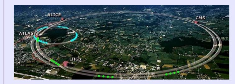
The Large Hadron Collider (LHC) in Geneva, Switzerland, is the most powerful collider built to date. It consists of two proton rings that run to collide in four different interaction points, including one where the CMS experiment is located.
