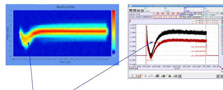
Beam energy and position in the transfer line varies over the first  $\sim$ 50 µs due to the beamloading transients in all RF cavities.
