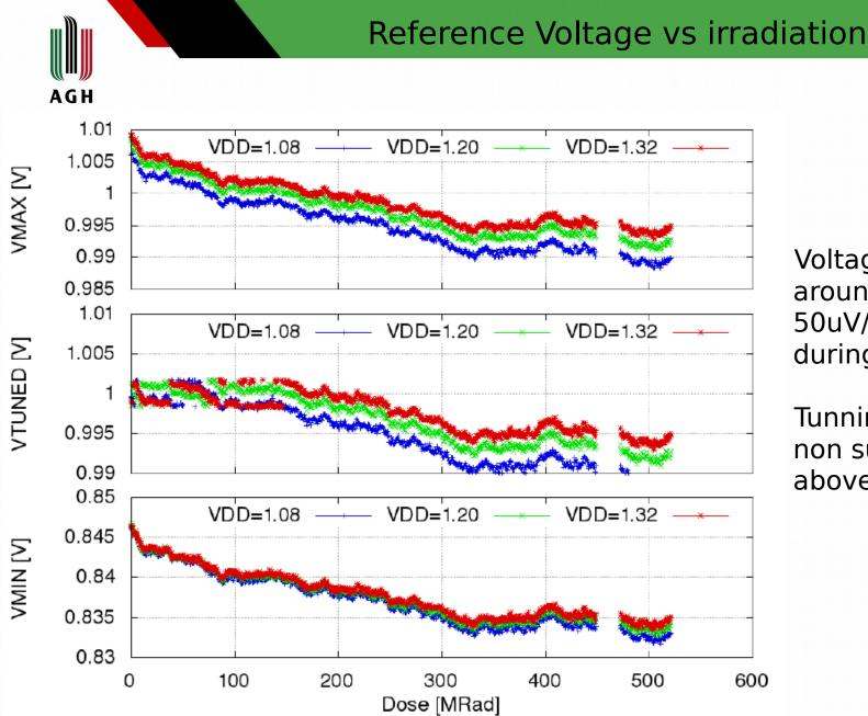
Voltage drops around 50uV/Mrad during irradiation
