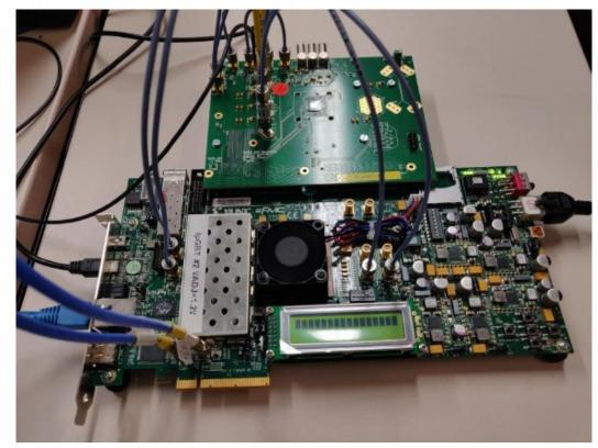
Dedicated FPGA-based measurement system, for more details see "LpGBT Tester: an FPGA based test system for the lpGBT ASIC" by J. Mendez et al.
