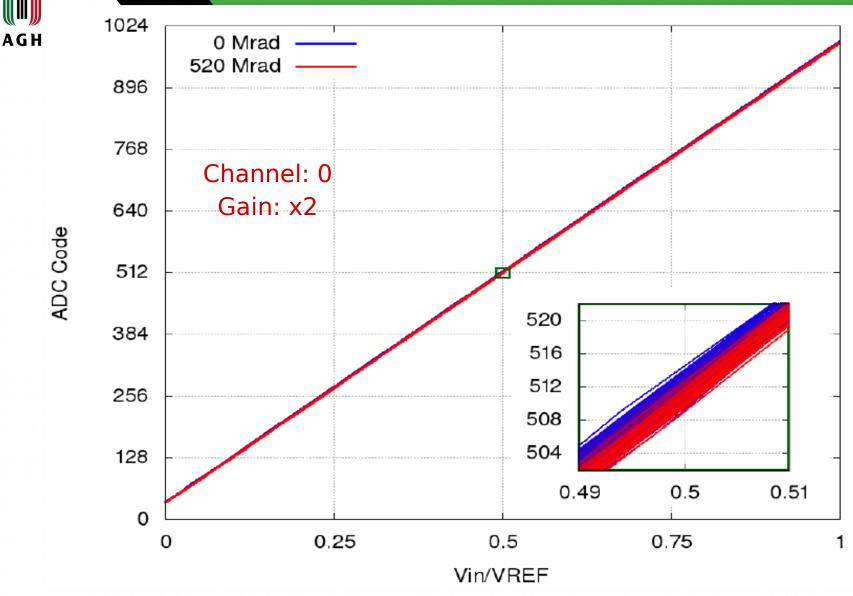
ADC linearity is very good up to 520 Mrad. No change during irradiation
