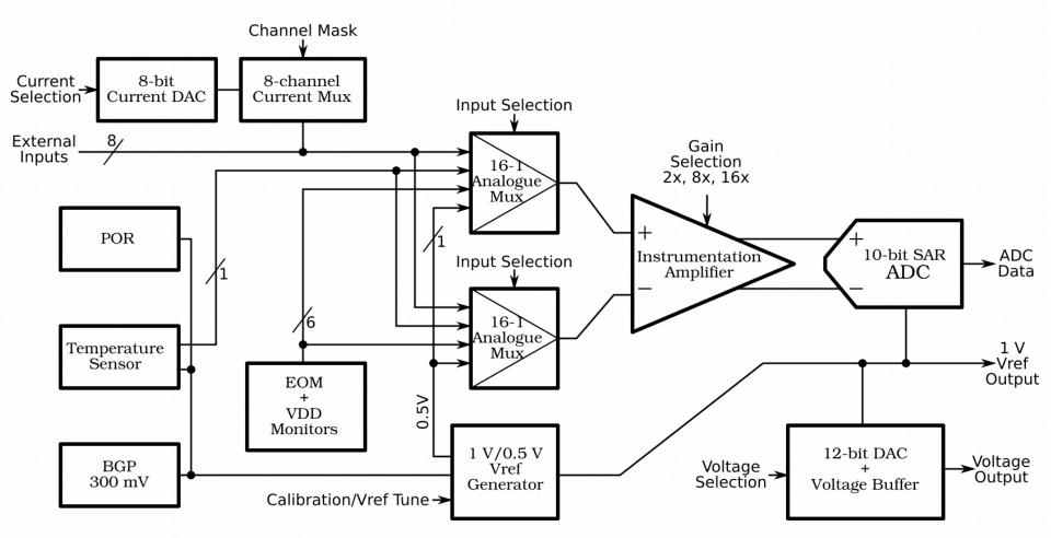
Block diagram of monitoring sub-system
