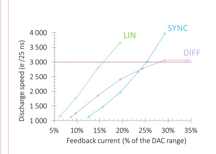
The discharge speed of the preamplifier can be modified by varying the feedback current. It is evaluated by injecting 6000 e<sup>-</sup> to each pixel and then dividing this charge by the mean time over threshold (unit: e<sup>-</sup>/ns).
