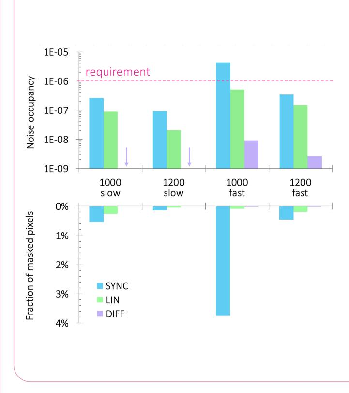
A million triggers is sent, with no charge injection and all pixels with 100 hits or more are masked. Then another million triggers is send, to estimate the noise occupancy after masking.
