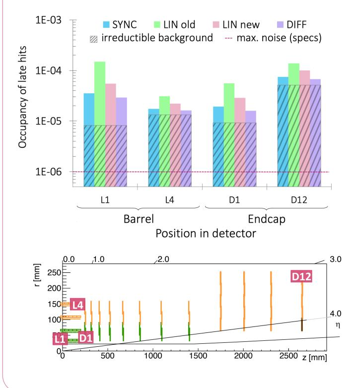
The time response of the front end is measured by injecting different charges with different time delays and checking whether the hit was found in a given time window. The occupancy of late hits is then obtained by combining the time response with time of arrival of particles from simulation.
