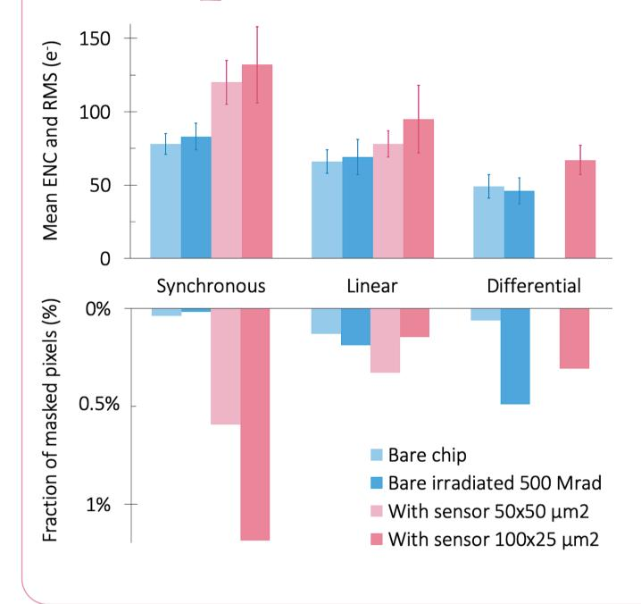
A million triggers is sent, with no charge injection and each pixel having at least one hit is masked. The equivalent noise charge (ENC) is then evaluated for remaining pixels from the slope of the S-curves.
