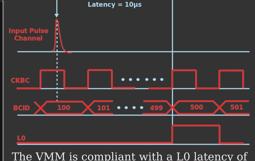
The VMM is compliant with a L0 latency of 10µs and a L0 rate of 1MHz for Phase-II, for a worst case scenario rate of 20 kHz/cm<sup>2</sup>
