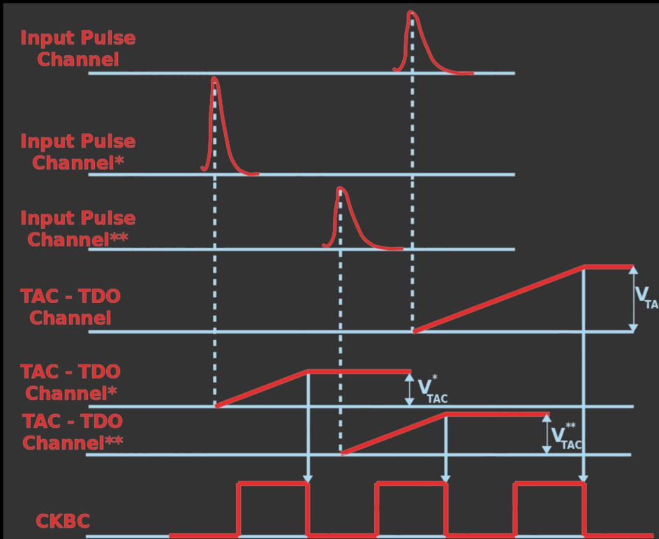
The channel's peak detector measures the pulse's amplitude, while the Time-to-Amplitude Converter (TAC) measures the timing of the pulse by using a voltage ramp that triggers on the pulse's peak (or at the threshold crossing) and halts on the next falling edge of the BC clock (see figure on the left). The two voltages are digitized by a set of innovative low-power ADCs [3]. The ADC data alongside the channel ID and the pulse's BCID tag are then stored in the VMM's L0 buffers
