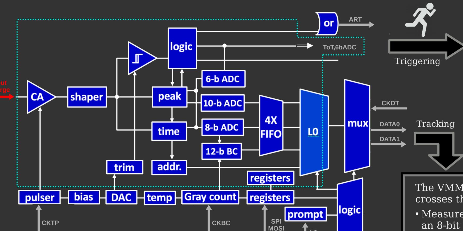
The VMM can be used for **Triggering**. Upon the detection of a peak that crosses the user-defined threshold, the chip:
